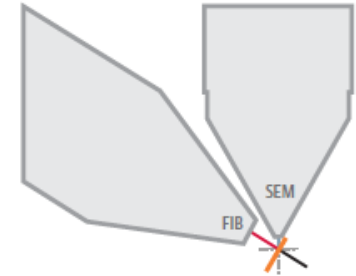
In a DualBeam™ the electron and ion beams intersect at a 52° angle at a coincident point near the sample surface, allowing immediate, high resolution SEM imaging of the FIB-milled surface.
