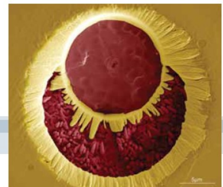
FIB-cut in steel v2a EE by InA to IB milling-002 steel.
