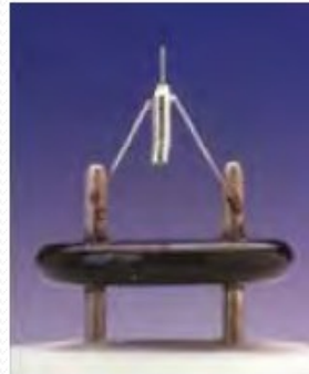
A FIB's liquid metal ion source (LMIS).
