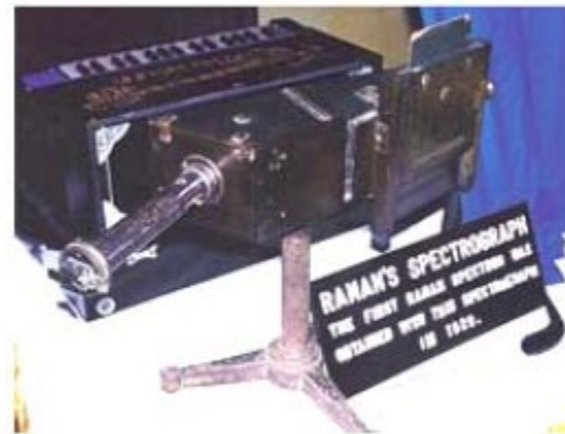
Raman's Spectrograph with Photographic Plate and 1st Spectra Published in Indian Journal of Physics
