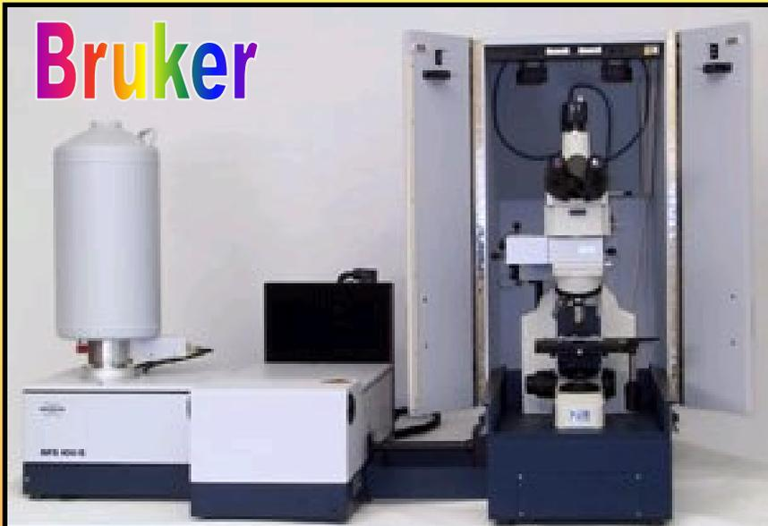
*RFS 100/S and RamanScope*
