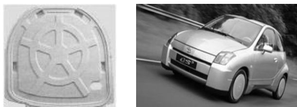
Fig. 6. TOYOTA „Ecoplastic“ Tire Cover in „New Raum“ Model 9
