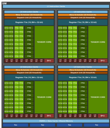
Figure: Ampere SM diagram. @ docs.nvidia.com
