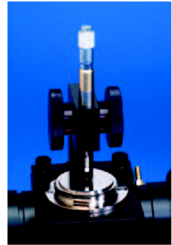
MIRacle Micrometer Clamp – OK for Low Pressure Applications
