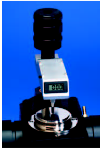
MIRacle Digital Clamp Ideal for Controlled Pressure
