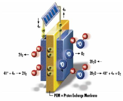
Fig. 1 Scheme of a PEM electrolyser.
